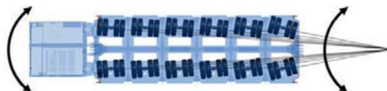
7. Transverse steering front/rear
