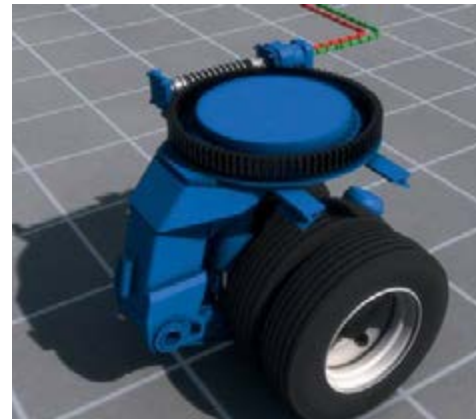
Electronically steered wheel set
