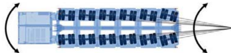
7. Transverse steering front/rear
