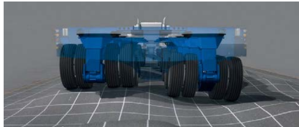
Hydraulic axle suspension – lateral + lateral swing movement
