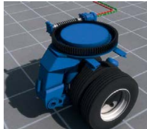
Electronically steered wheel set
