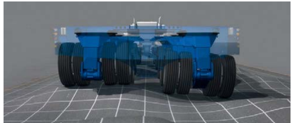
Hydraulic axle suspension – lateral + lateral swing movement
